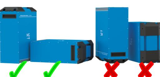
Leave a **minimum space of 10 mm** all around the battery including the bottom side lifted from the surface. Secure the battery with a strap or a bracket.
